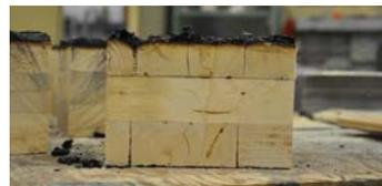
assemblies of non-combustible construction. This is due to the inherent nature of thick timber members to char slowly at a predictable rate, allowing massive wood systems to maintain significant structural capacity for extended durations when exposed to fire.
