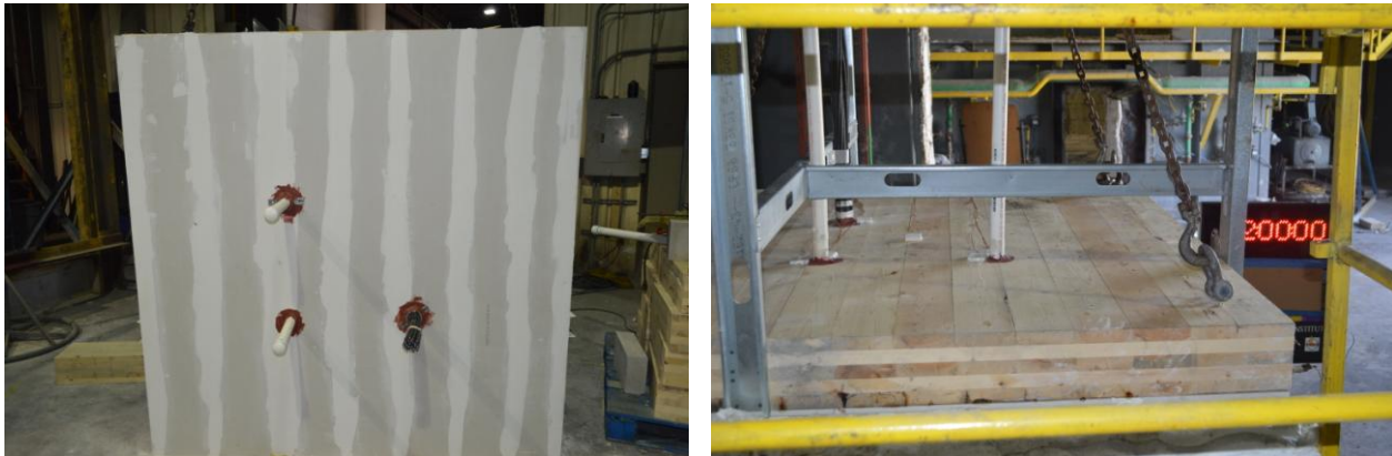
Figure 1: Test Assembly with Through-Penetrations.
