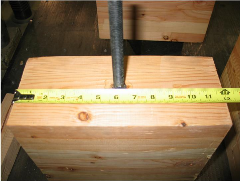
Figure 1: Glulam test specimens with threaded rod exposed.
